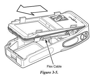
5. Pull the chassis out and away from the housing as shown by the arrow in Figure 3-5.
