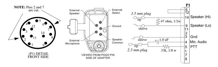
**NOTE:** For proper speaker impedance, the RTX4005B test set *Audio out* switch must be set to the **"MX"** position
