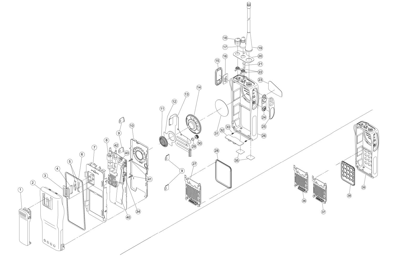
Exploded Mechanical View and Parts List (Basic)
