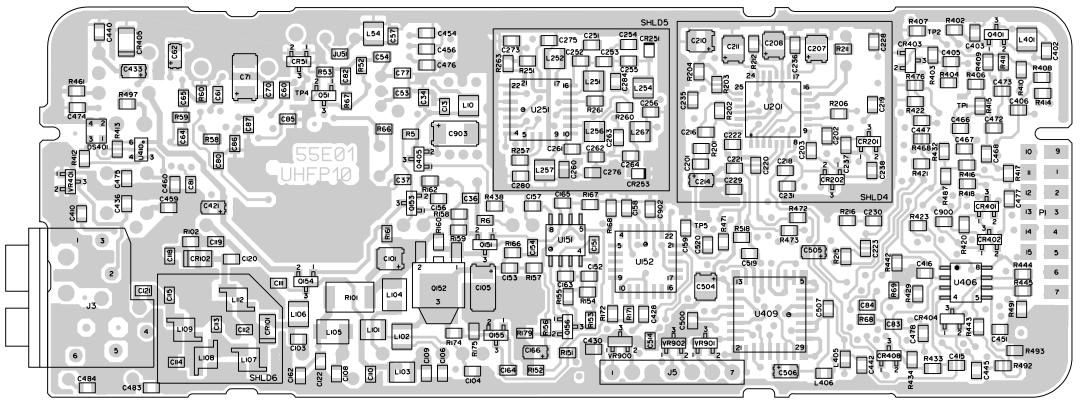
Component Location Diagram for HLE9480A and HLE9481A UHF, 438-470MHz, Transceiver Section
