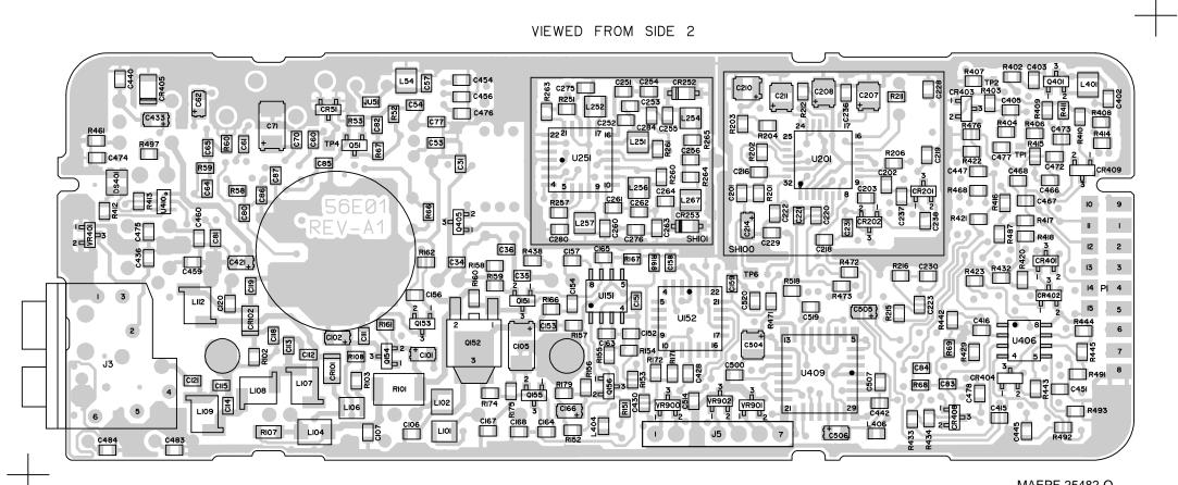
Component Location Diagram for HLD9440A and HLD9441A VHF, 146-174MHz, Transceiver and Controller
